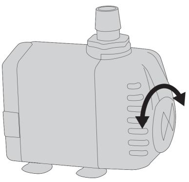
For models PHX 150/200/300, the flow rate can be adjusted using the valve on the intake strainer as shown.
